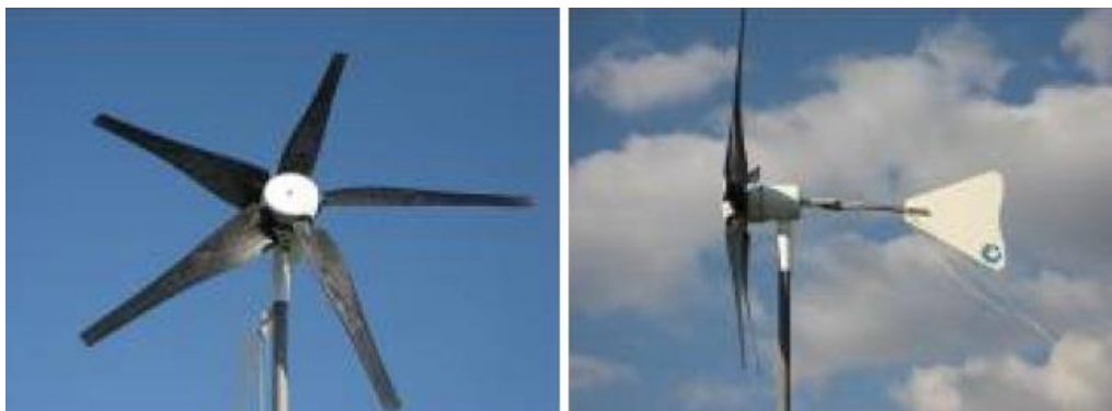
Figure 8 - Turbine faced at 0 and 90 degrees (respectively) to the radar
