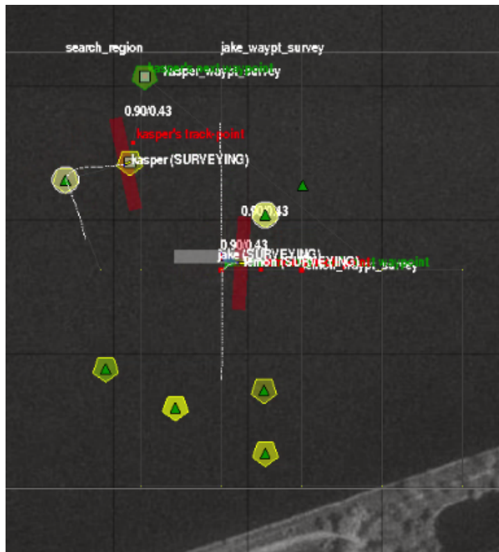
Figure 5.6: Mismatch in the synchronous rendezvous time and vehicle paths. The problem is due to the merged reports which did not get synchronised. Some vehicles calculated their path and SR based on a partial report. This happens when a message does not get through or when a vehicle is late to arrive at the SR.
