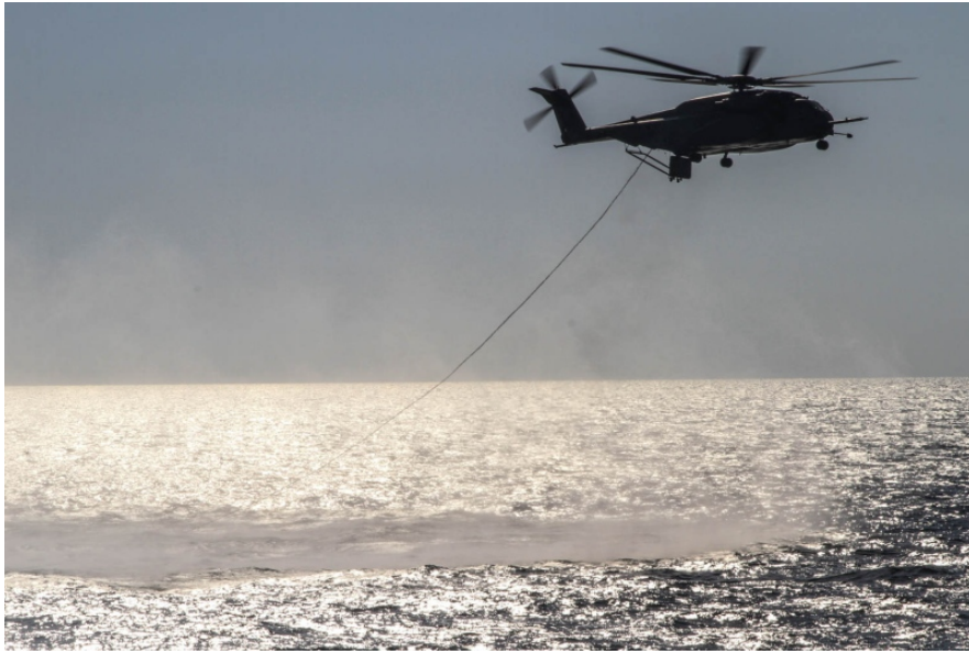
Figure 1.12: An MH-53 helicopter, during a mine sweeping exercises in the Persian Gulf in 2014 - equipment that cuts the chains off sea mines is towed and the mines are revealed by floating to the surface 6
