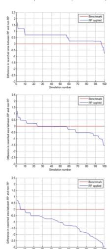
number of contacts, the RP gives a significant gain over the benchmark case in the majority of the simulations, even though the loss for vehicles meeting is accounted for. It is obvious that this is the most advantageous situation to apply RP.
