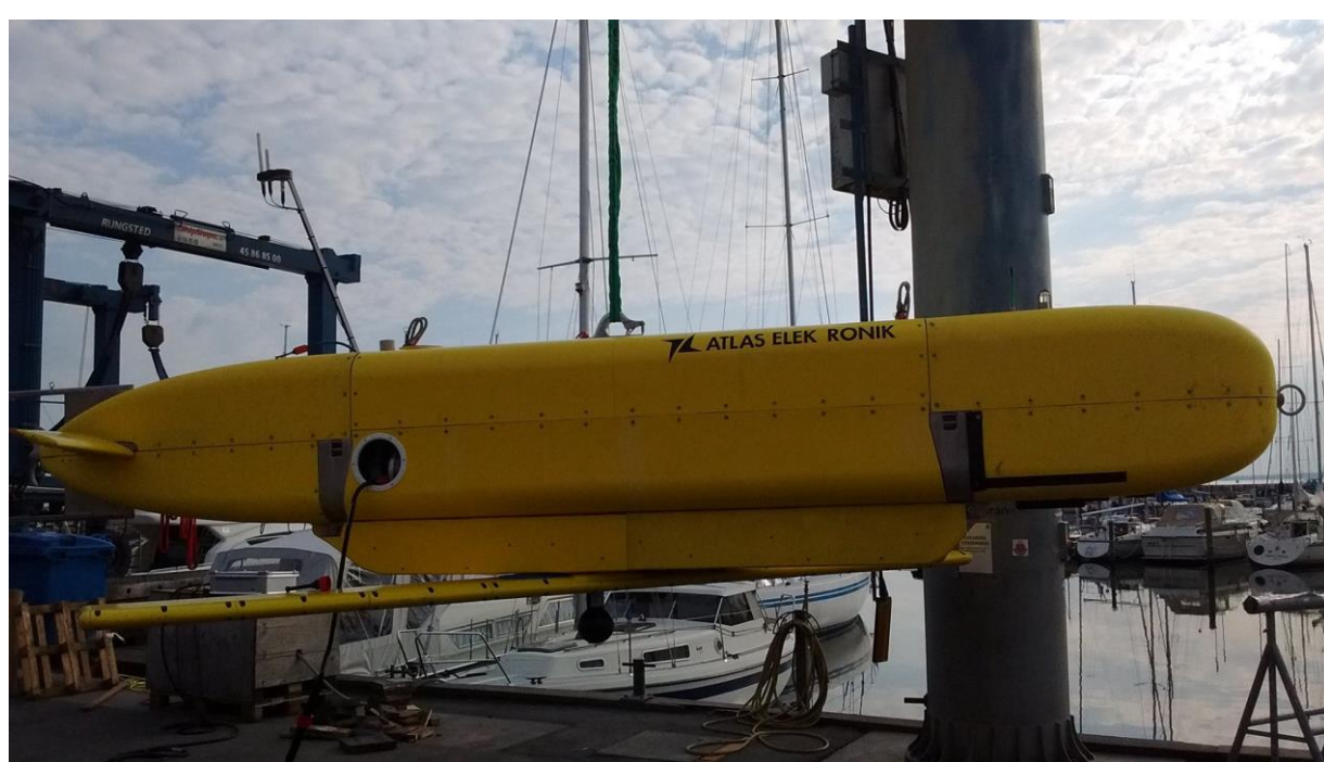
Figure 1: Capitas AUV equipped with a side scan sonar used for field experiment in the North sea at the coast of Denmark
